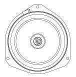
Place the new DLS Cruise driver in the hole for the original speaker. Use the OEM screws to safely mount the driver.
