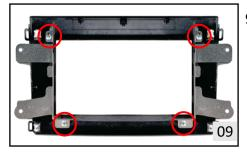
Fix the metal brackets to the facia plate by tightening the 4 screws (2 per side) supplied in the kit.
