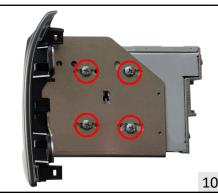
Fix the facia plate to the radio by tightening the 8 screws (4 per side) supplied in the kit.
