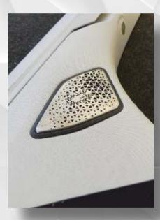
The finished fairing can be reinstalled in the vehicle. Please make the cable connection of the new tweeter unit with the original cable of the vehicle.
