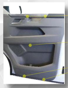
In the yellow marked fields there are fasteners that need to be loosened.
