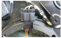
Glue the supplied sealing rings to the back of the new speaker rings. This is now attached to the door carrier with the metric screws and nuts. Connect the enclosed cable adapter with the original connector plug and insert it into the recess on the speaker ring.
