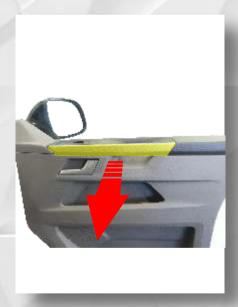
To remove the door trim, use a plastic tool to click out the upper handle trim. There are two fastening screws under this.
