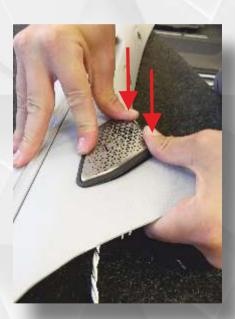
Carefully press the tweeter unit into the grille with light pressure until it snaps firmly into place.
