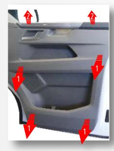
Pull off the door trim using a plastic tool (step 1) and then unhook it from the upper window seal (step 2).
