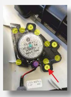
To remove the original tweeter and front grille, the plastic welds marked in yellow must be loosened.
