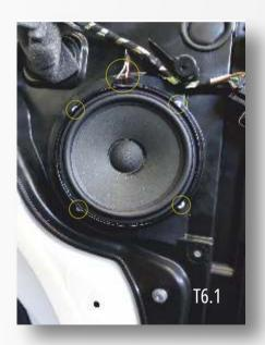
To disassemble the original speaker, please disconnect the connector plug. Then the fastening rivets on the speaker must be drilled out.
