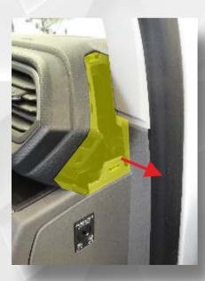
Use a plastic tool to carefully loosen the trim below the A-pillar. This is clicked into place with retaining clips. (Only T6.1)
