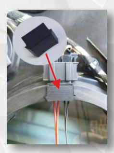
Insert the sealing pin shown in the picture into the speaker ring. This serves to fix the cable adapter.
