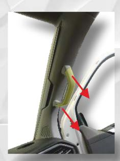
To remove the A-pillar trim, click out the upper handle trim with a plastic tool. You will find a recess below the handle for this purpose.
