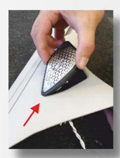
Insert the tweeter insert, pointed side first, into the opening in the panel.
