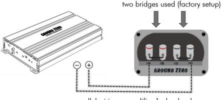
parallel wiring – amplifier 1 ohm load
