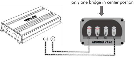
serial wiring - amplifier 4 ohm load
