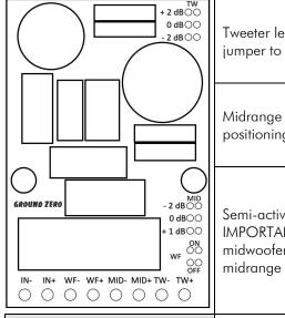
Tweeter level adjustment: The tweeter level can be set by positioning the jumper to the required level position
