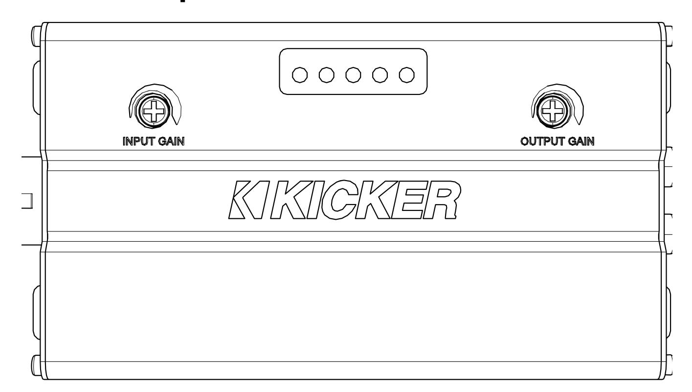
After Auto Setup is complete, use the Output Gain to match the output voltage of the KEYLOC to the input sensitivity voltage of your amplifier. If you're not using gain match capable electronics or a voltmeter/multimeter, listening for audible distortion is always the next best way to set your gain.
