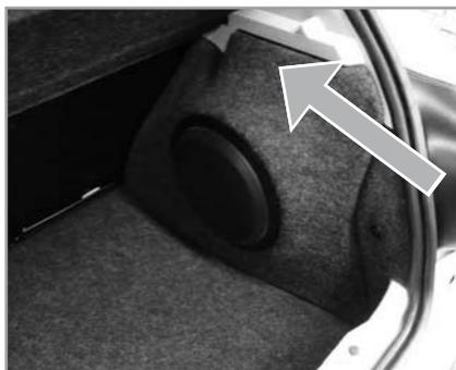
Set in the enclosure to its final position and press it tightly against the vehicle interior wall, that both hook and loop stripes are firmly connected.
