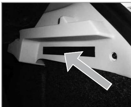
Stick one part of the included hook and loop tape to this position in the trunk.
