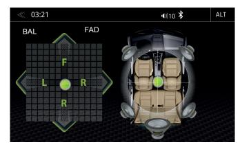
In this Expert Mode menu page, you can adjust the balance and faders. Press and hold the green dot of the crosshair to move sound center position into any desired position.
