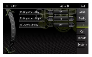
In the TFT Setup menu you can make screen settings that control the day/night brightness of the TFT LCD display screen.
