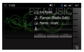
The A2DP RVC interface offers Play, Pause and Skip control of previously paired smartphones in audio playback mode. The iD3-Tag meta data display is possible only when tag data is contained in the streamed music track.
