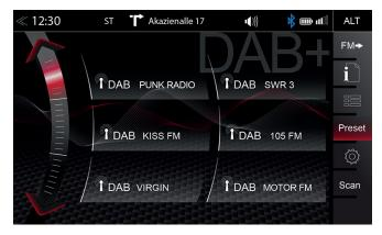
Select a previously stored DAB+ radio station by tapping on the station preset button.
