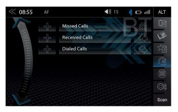
If a compatible mobile phone is connected, call lists from the mobile phone will be synchronized with the BT hands-free system (process can take some minutes, depending on the number of contacts). Once sync process has completed you will be able to access the following logs:
