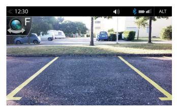
Tapping the camera icon starts the manual camera mode, if a CVBS capable camera is connected to the camera input of the unit.
