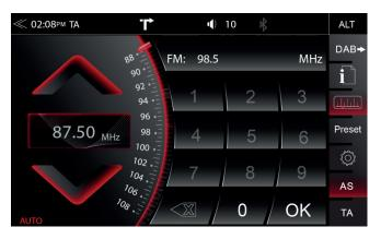
When you tap to the frequency display area, the numeric input keyboard opens for a direct station frequency input.
