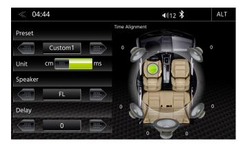
In this menu you can set the time delay correction for the loudspeakers in your vehicle.
