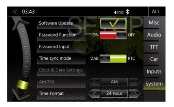
In the System Setup menu page under Clock Time, you can set the format, change the displayed time and select the time sync source (system time or DAB) for the time display.
