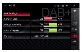
The setup page for the DAB+ tuner allows to define important functions such as DAB<>DAB service following. Or to activate the phantom power supply voltage of the DAB antenna socket.
