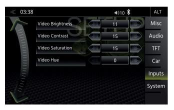
In the Input Setup menu, you can adjust the image settings of the connected video sources, such as Reverse Cameras. Contrast, brightness, color saturation and hue can be adjusted.
