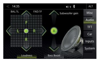
In this menu, you can adjust the Balance / Fader, Loudness and Subwoofer level of the speakers in the vehicle.
