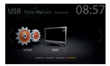
With the display icon, the LCD TFT screen picture brightness can be dimmed or switched off (standby) in two steps. This is done by tapping the icon.
