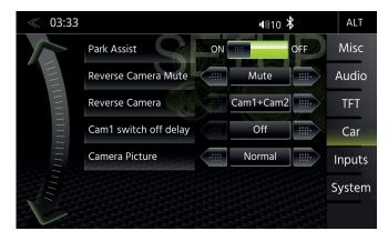
In the Car Setup menu, you can set how the ZENEC device interacts with optional components such as cameras and parking assist inside the vehicle.
