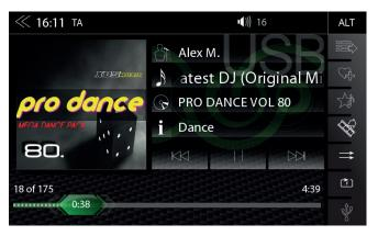
Various types of information shown in the source menu of the audio playback by (USB, BT A2DP, iPOD, etc.).
