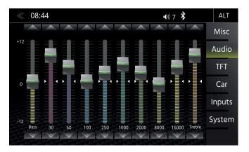
In this Expert Mode menu page, you can set the 8-band graphical equalizer. Press and hold the individual band level sliders to move it up or down for a level change.
