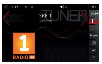
The FM RDS source menu offers a control-/operating section on the right hand side, for fast and convenient adjustments during the FM radio playback.
