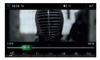
For video playback via USB, parking cable must be connected during the device installation. Without this connection, the screen remains black.
