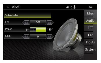
In this Expert Mode menu, you can adjust Phase, Gain, and Low-pass transition frequencies of the subwoofer. The default settings are Phase 0  $^{\circ}$ , GAIN "0", LPF OFF.
