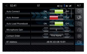
On the Bluetooth setup page you can adjust settings for Bluetooth operation. Press the appropriate button / field to change any of the listed settings.
